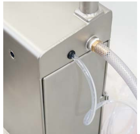
Separate supply of the cleaning detergents
