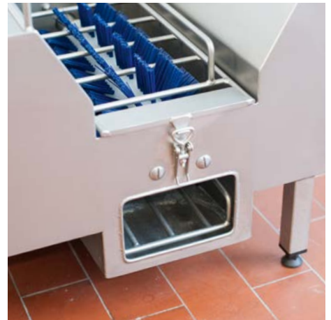
Separate cleaning of sole and upper shoe
